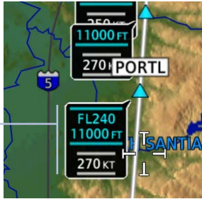
Altitude Constraint Label with Speed Constraint
