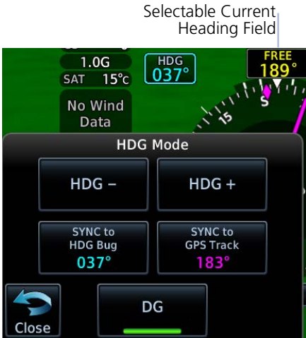
“FREE” annunciates above the current heading value when DG free mode is active. “HPM” annunciates when HPM mode is active.
